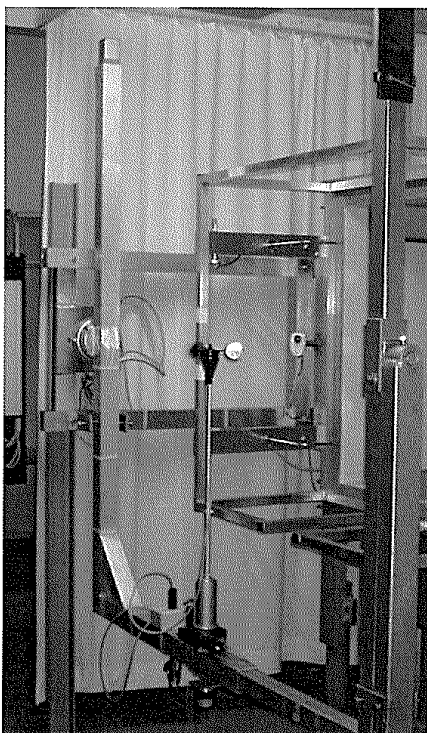
Calibration set-up of the anemometer calibration in the wind tunnel of Deutsche WindGuard, Varel. The anemometer shown is of the same type as the calibrated one. Remark: The proportion of the set-up are not true to scale due to imaging geometry.
