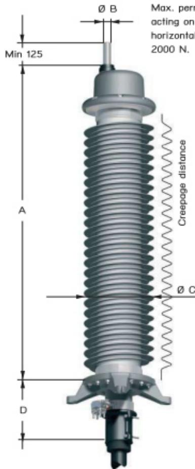
Max. permissible forces acting on the top bolt, horizontally and vertically: 2000 N.
