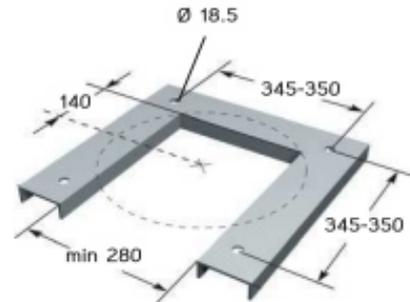
Fixing to bracket for 420 kV
