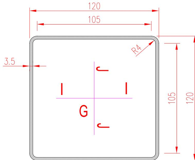
*Inertia Characteristics (dimensions in mm)*
