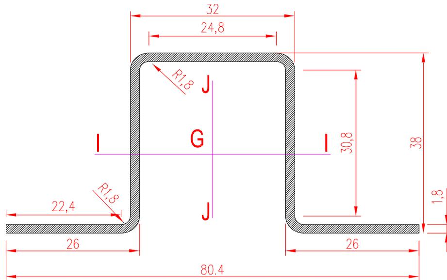
*Inertia Characteristics (dimensions in mm)*
