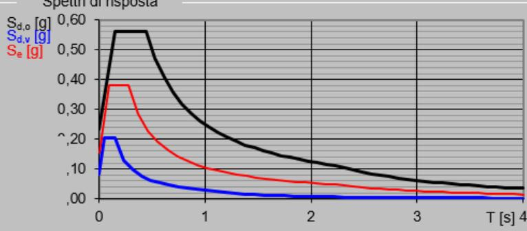
The graph plots acceleration in g against period T in seconds. The horizontal component (black line) peaks at approximately 0.55g around 0.2s. The vertical component (blue line) peaks at approximately 0.20g around 0.1s. The reference elastic spectrum (red line) peaks at approximately 0.38g around 0.1s. The x-axis ranges from 0 to 4 seconds, and the y-axis ranges from 0.00 to 0.60 g.
