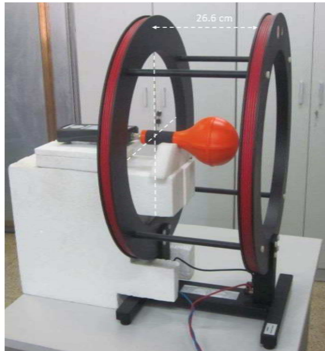
Figure 2: Calibration set-up in the Helmholtz coils system – B field
