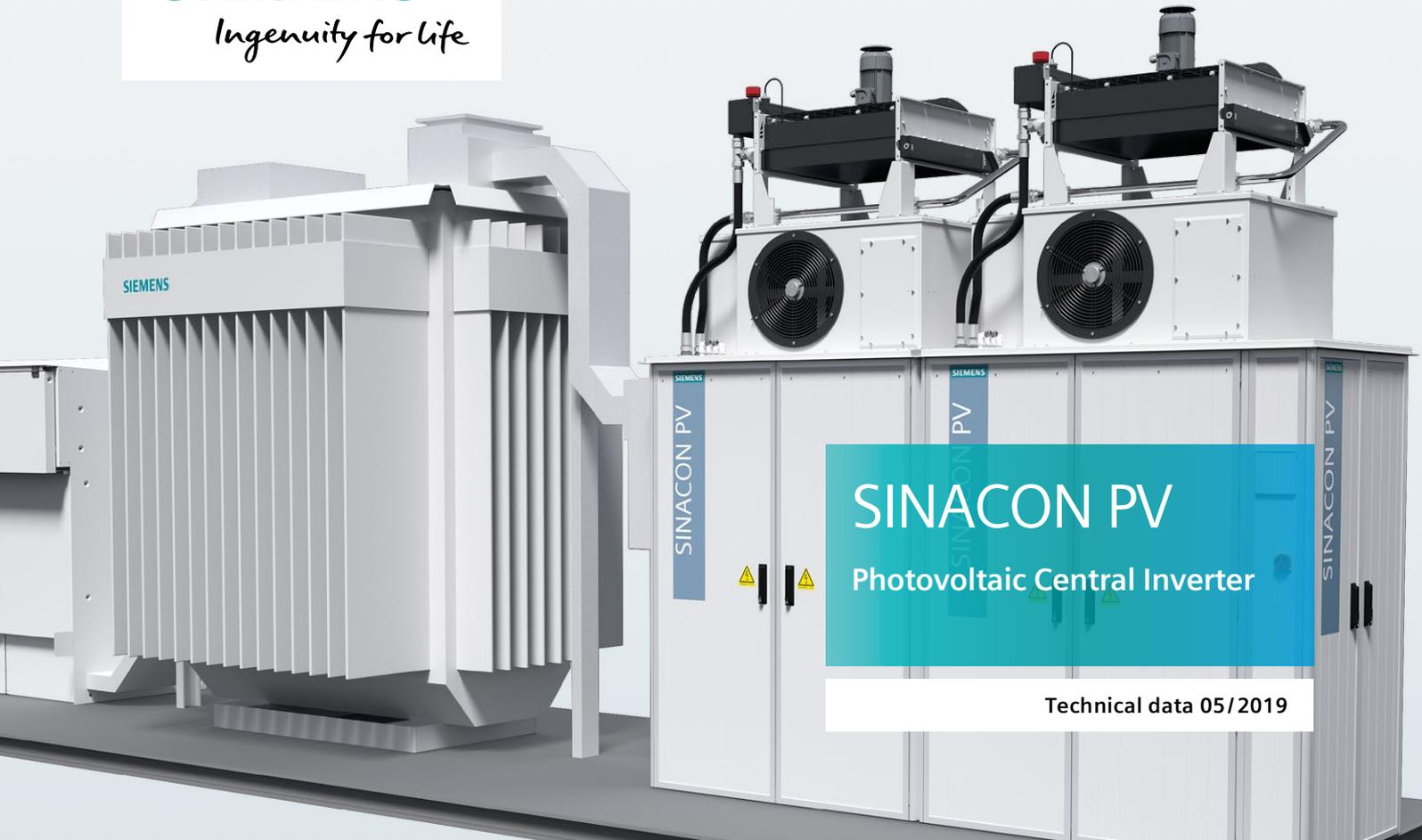
The SINACON PV inverter is used in medium and large utility-scale photovoltaic power plants to achieve high efficiency. It is equipped with 3-level IGBT modules for input voltages of up to DC 1500 V to maximize energy efficiency. The integrated DC and AC distribution makes the SINACON PV inverter cost efficient. Standardized interfaces for easy plug and play reduce engineering hours.
