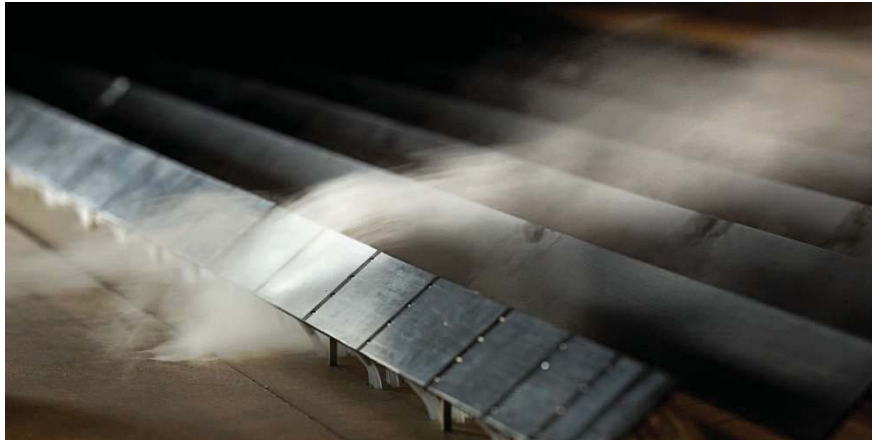
Wind tunnel test studies of PV array allow optimizing the tracker structure
