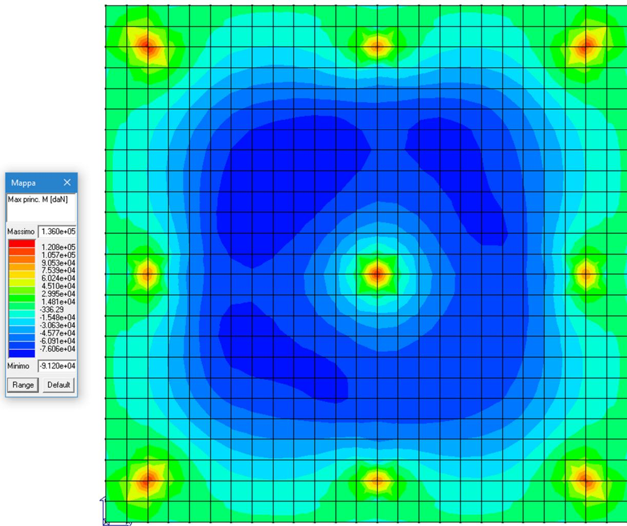
*Figura 9 – Von Mises: Max princ. M (daN)*
