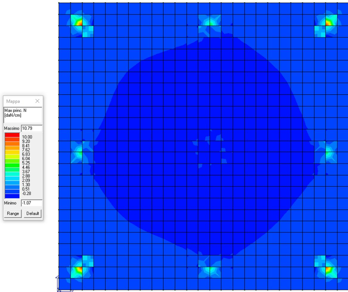
*Figura 8 – Von Mises: Max princ. N (daN/cm)*
