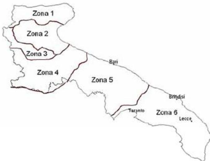
$$\begin{aligned} \text{Zona 1: } & x(t,z) = 26.8 t^{\{(0.720+0.00503 z)/3.178\}} \\ \text{Zona 2: } & x(t) = 22.23 t^{0.247} \\ \text{Zona 3: } & x(t,z) = 25.325 t^{\{(0.0696+0.00531 z)/3.178\}} \\ \text{Zona 4: } & x(t) = 24.70 t^{0.256} \\ \text{Zona 5: } & x(t,z) = 28.2 t^{\{(0.628+0.0002 z)/3.178\}} \\ \text{Zona 6: } & x(t,z) = 33.7 t^{\{(0.488+0.0022 z)/3.178\}} \end{aligned}$$
