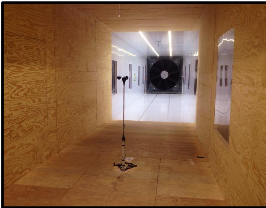
Photo of the wind tunnel setup. The cross-sectional area is 2.5 \text{ m} \times 2.5 \text{ m}
