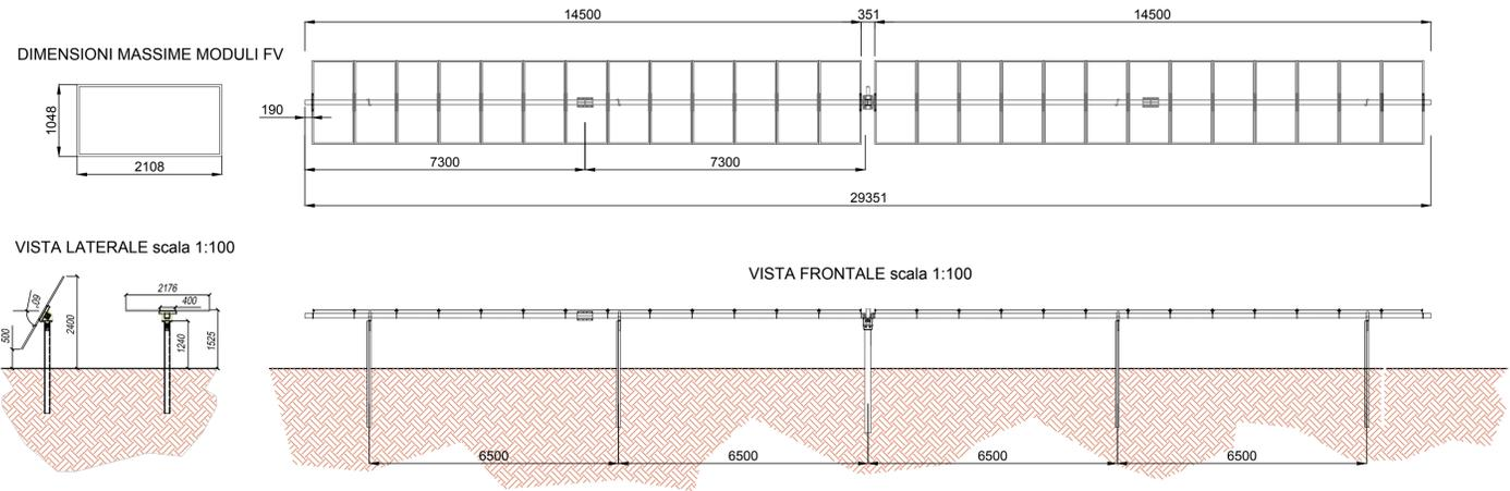
TIPO TRACKER DI SUPPORTO MODULI FOTOVOLTAICI
