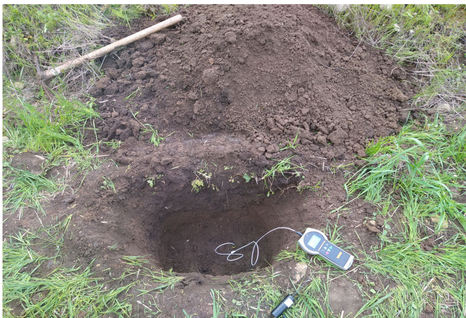
Misura RESISTIVITA' TERMICA (ASTM D 5334-14) RESTER04
