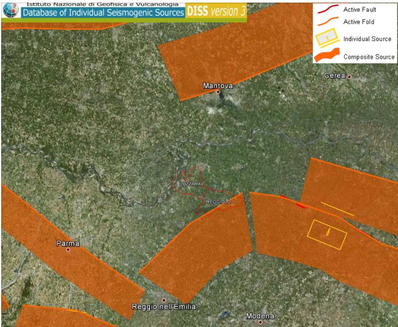
**FIGURA 6-1: SORGENTI SISMOGENETICHE CONTENUTE NELLA NUOVA VERSIONE DEL "DATABASE OF POTENTIAL SOURCES FOR EARTHQUAKES LARGER THAN M 5.5 IN ITALY" PER L'AREA IN OGGETTO**
