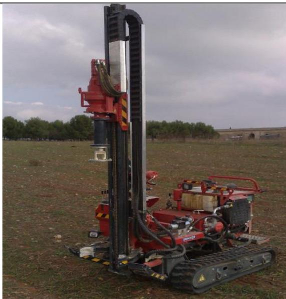
**FIGURA 8 - MACCHINA BATTIPALO PER INFIESSIONE PALI.**
