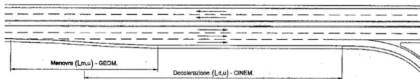
**FIGURA 3.2-3 - SCHEMA PLANIMETRICO CORSIE D'USCITA PARALLELE**
