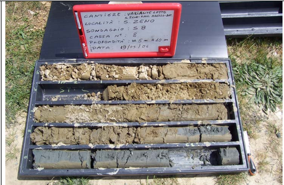
Sondaggio 8 – cassa n° 2 – da 5,0 a 10,0 m
