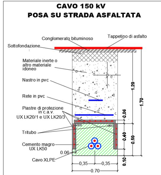
Figura 2: Posa cavo 150 kV "SE 30/150 kV – SE "Cancello 380"
