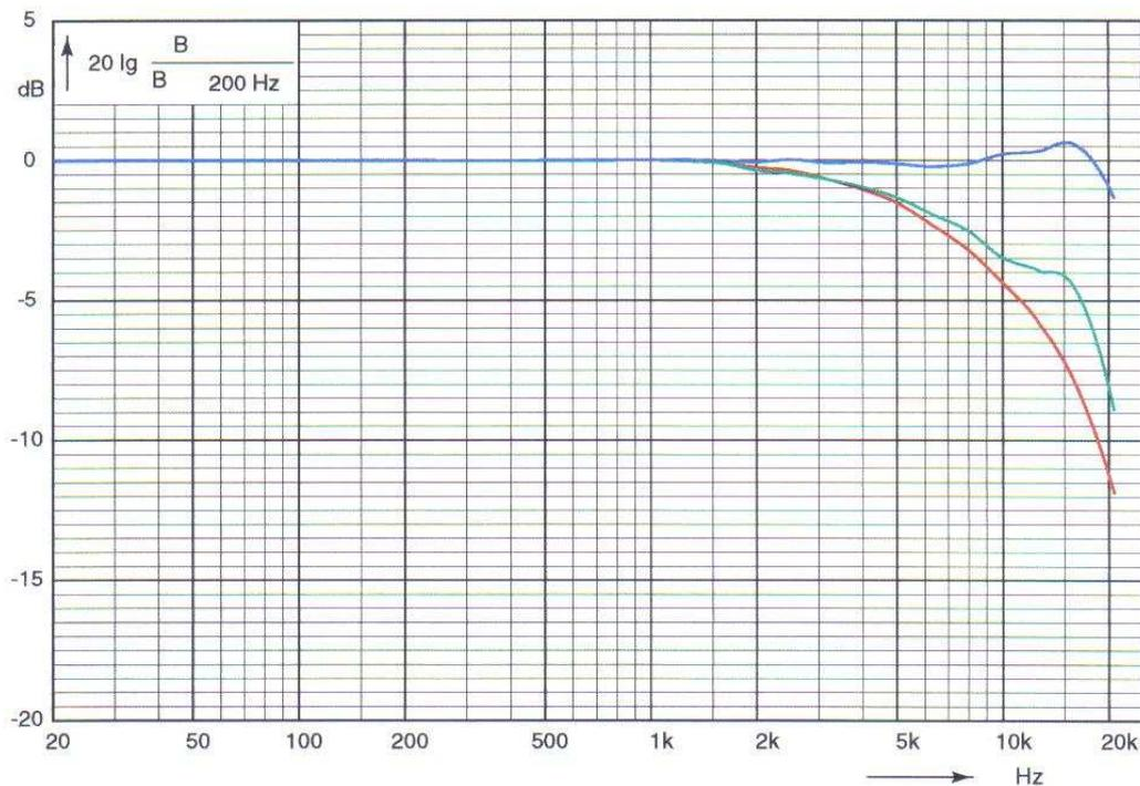
**Frequency response for microphone with protection grid**
