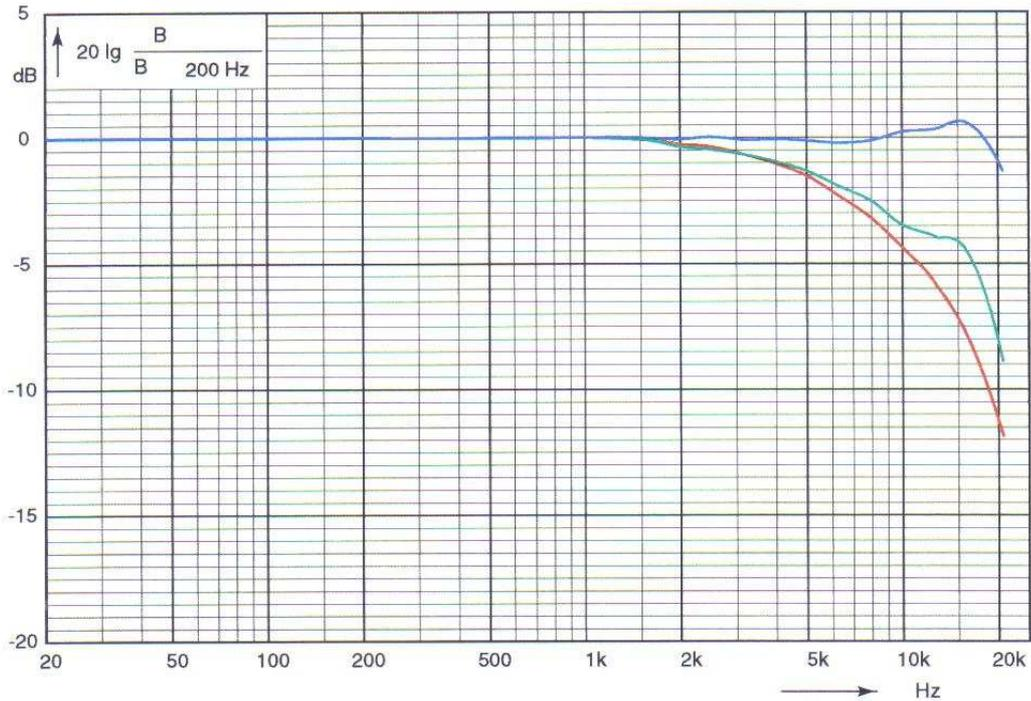
**Frequency response for microphone with protection grid**
