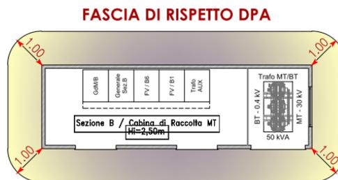
$$\left[ \begin{array}{l} \text{TRAFO 50 kVA} \longrightarrow I = 72 \text{ A} \\ \text{CAVI 1x35 mmq} \longrightarrow D_e = 14,6 \text{ mm} \end{array} \right]$$
