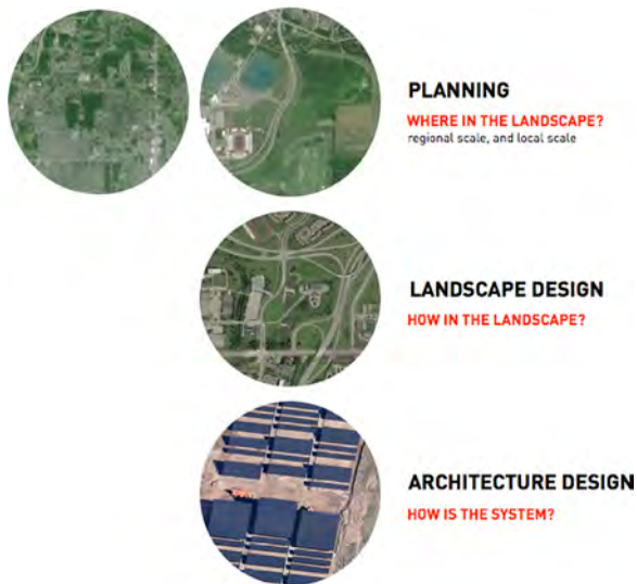
Fig. 12. Conceptualization of the main spatial design actions when implementing photovoltaic landscapes. The first level (regional and local scale) is the one of the planning, aimed to the site selection. The second level is the landscape design, whose object is the design of the photovoltaic landscape pattern. The third level is the architecture design, whose object is the design of the photovoltaic system. These design processes and associated choices are interlinked, spatially and temporally.
