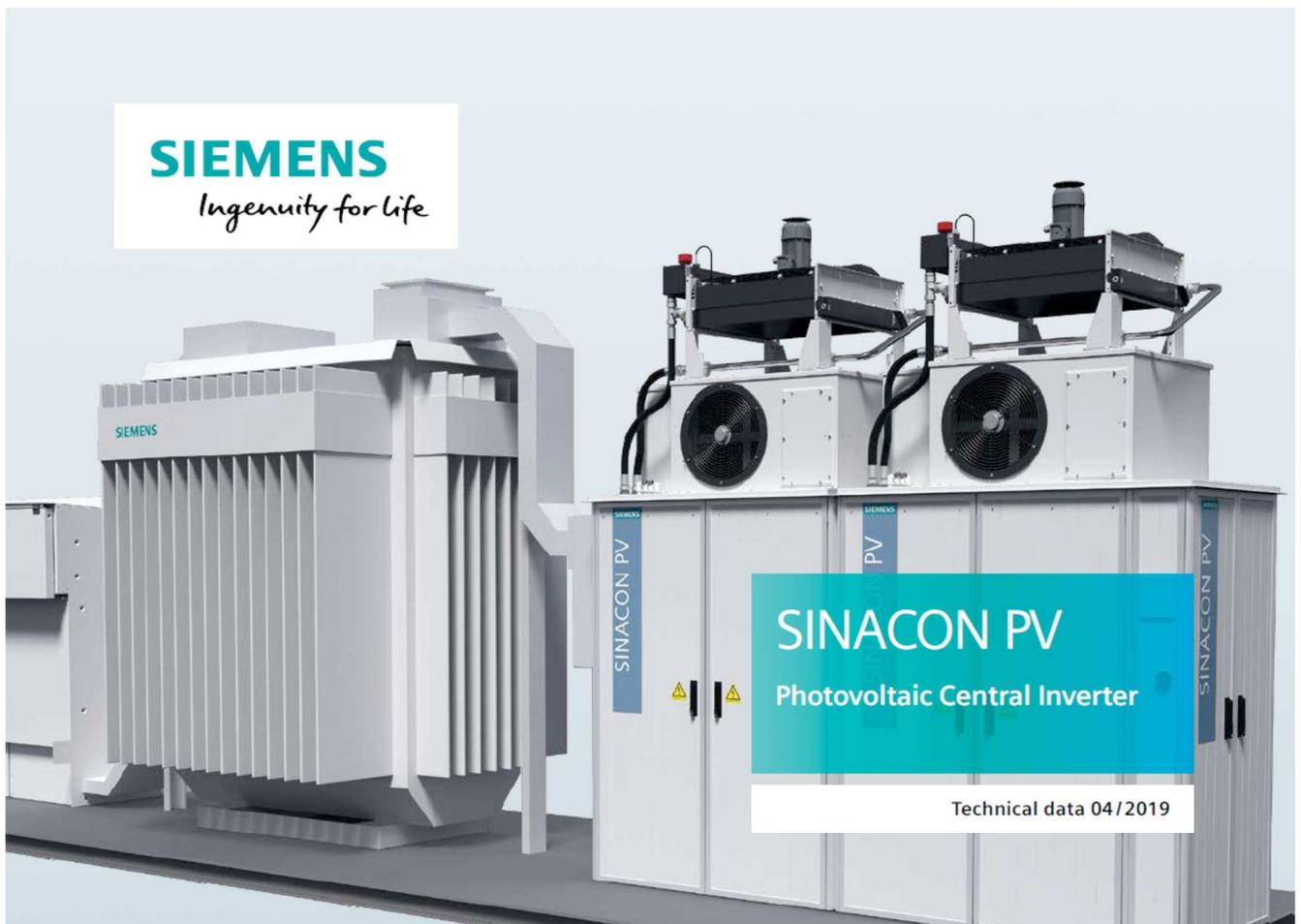
The SINACON PV inverter is used in medium and large utility-scale photovoltaic power plants to achieve high efficiency. It is equipped with 3-level IGBT modules for input voltages of up to DC 1,500 V to maximize energy efficiency. The integrated DC and AC distribution makes the SINACON PV inverter cost efficient. Standardized interfaces for easy plug and play reduce engineering hours.
