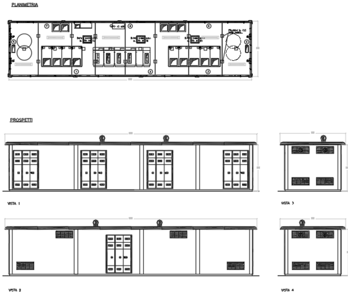
Figura 3.8 – Tipologico cabina Power Station.
