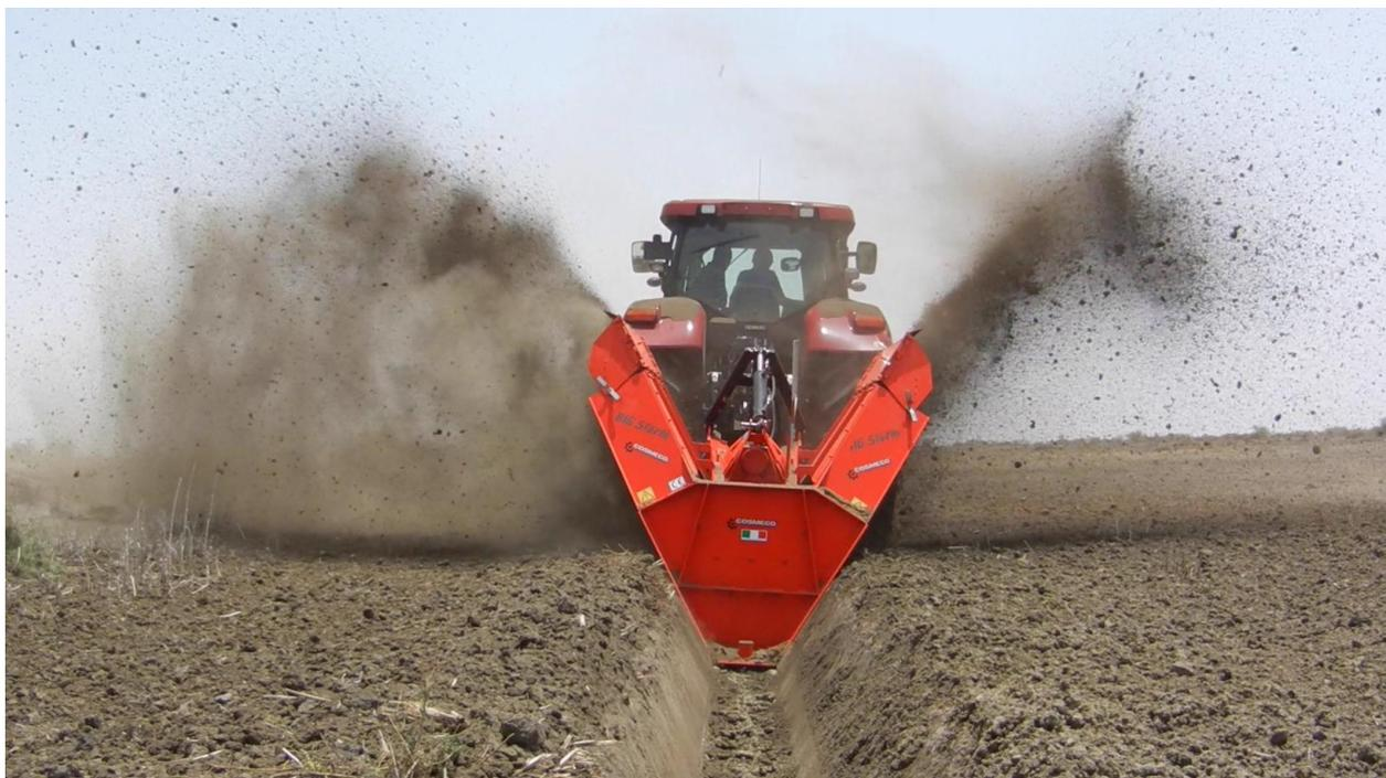
FIG. 12 - MACCHINA SCAVAFOSSI DEL TIPO ROTATIVA BIRUOTE
