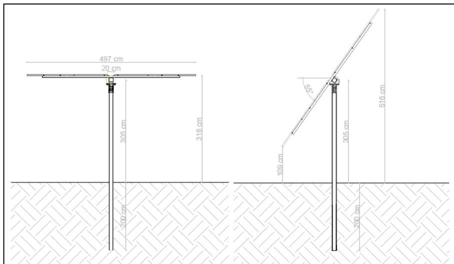
FIGURA 2: SCHEMA TIPO TRACKER AD ASSE VARIABILE
