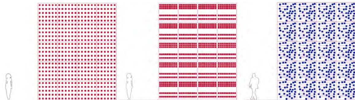
Fig. 3. Design possibilities for photovoltaic patterns, based on geometries: orthogonal grid, parallel stripes, random. A part from the type of pattern, it is possible to associate to each pattern a certain "density", that is the amount of elements in a given area. In the case of a photovoltaic pattern, the density, and therefore, the degree of "porosity" of the pattern is associated to the nominal power of the system (density of power, \text{kW}_p/\text{m}^2 ).
