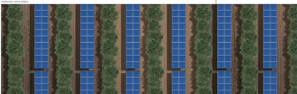
The trackers of the photovoltaic system will be interspersed with rows of olive groves.
