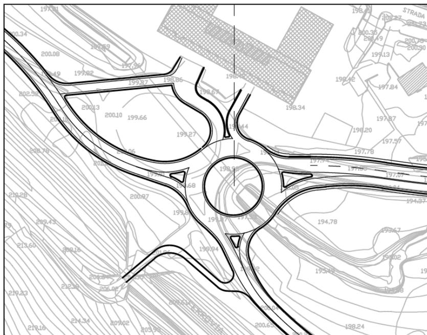
Figura 164 – SDP1 e SDP2: layout rotatoria INT 03
