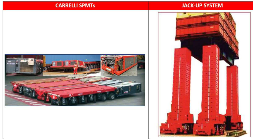
Figura 10-2 - SPMTs e Jack up system
