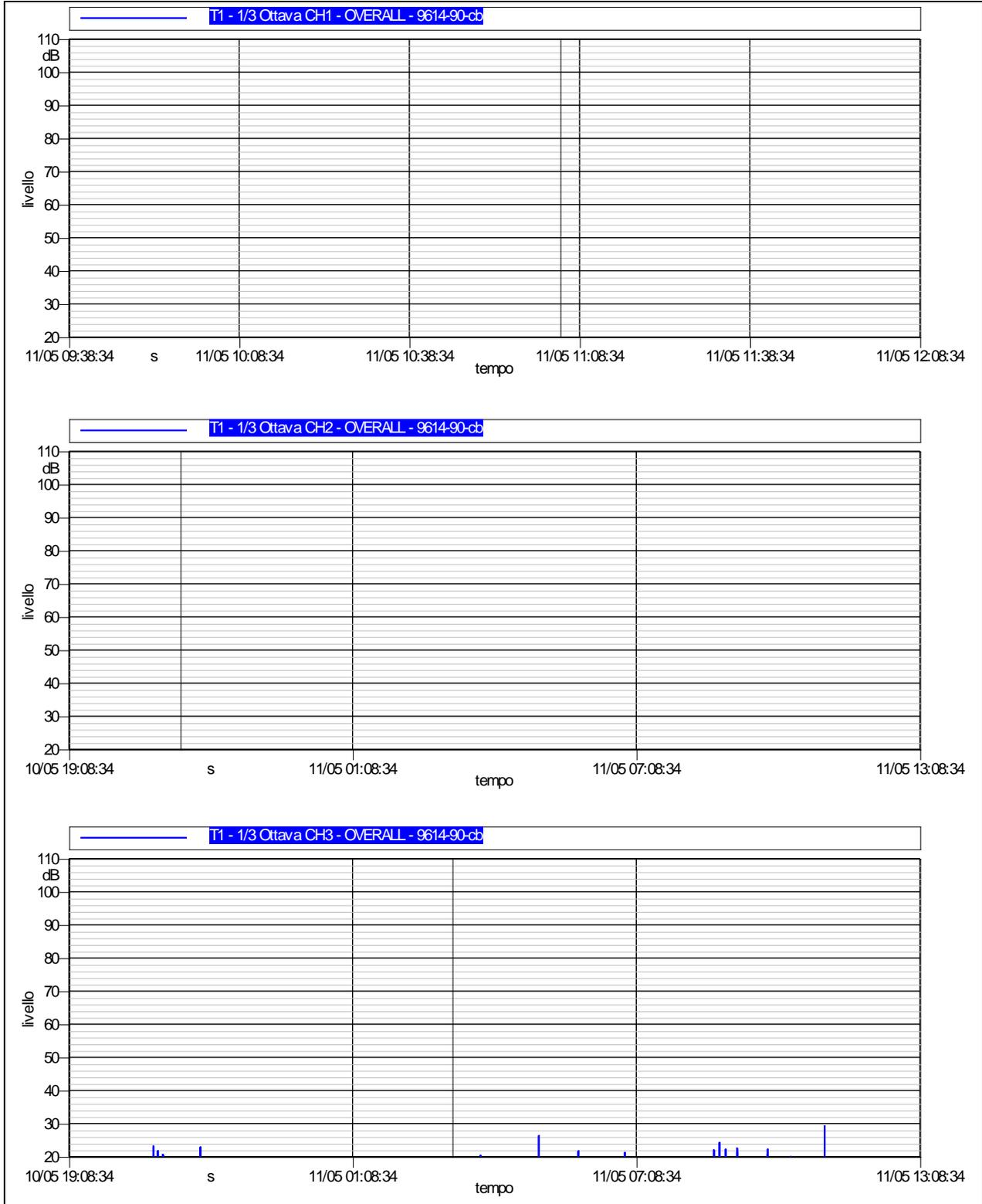
UNI 9614 ACCELERAZIONI R.M.S. – TERNA 2 CH1-X, CH2-Y, CH3-Z
