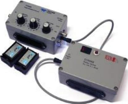
EC6081 mk2 can run on power from the old EC6068/ EC6069 or the old EC6072 supply when connected with the old TL8084 cable. Remove the rechargeable batteries first as the old EC6068/6069/6072 operates at 12VDC and 18VDC. EC6081 mk2 operates at 18VDC nominal (range min 10VDC to max 30VDC) but the charge circuit in EC6081 mk2 requires 24VDC.
