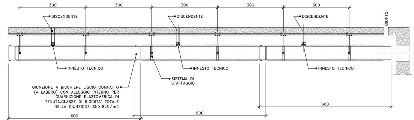
DETTAGLIO MARCIAPIEDE CON CADITOIA E COLLETORE DI RACCOLTA ACQUE DI PIATTAFORMA
