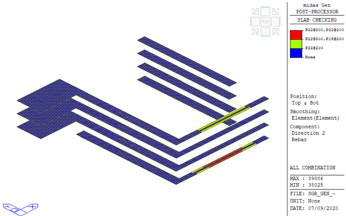
Figura 9.27 –Copertura armature dir.2 (asse y)
