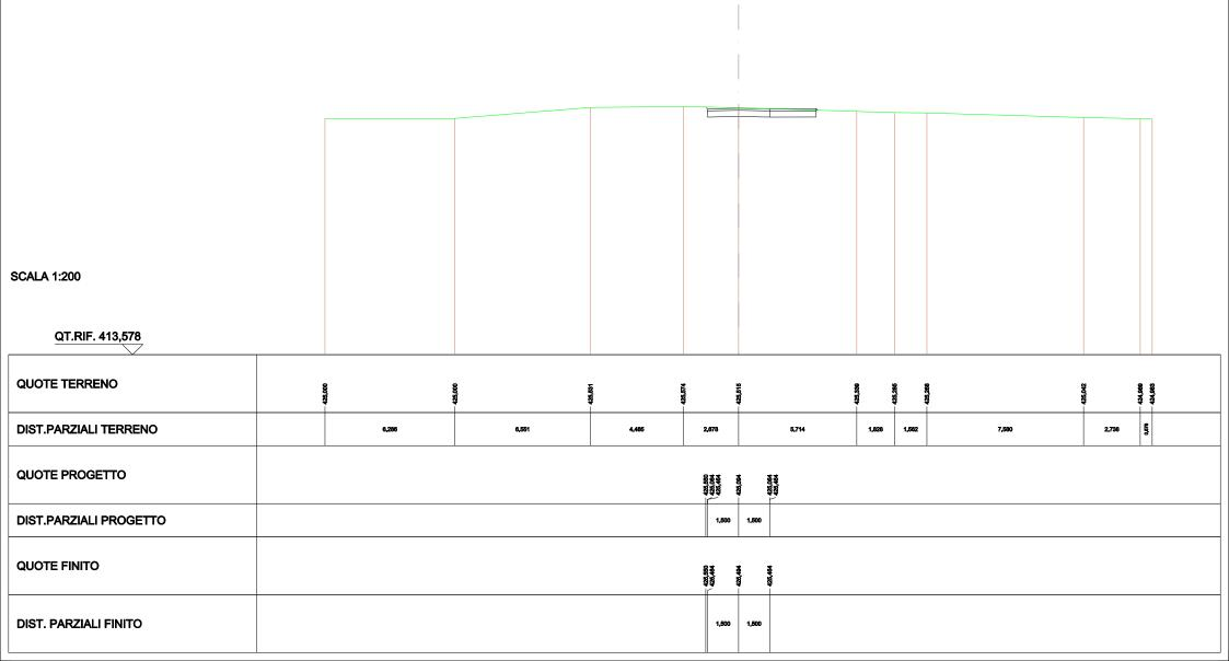
SCAVI E BONIFICHE STERRO RILEVATI SEZIONE N.: 5 QT. PROGETTO: 425,375 DIST.PROG.: 14,199 DIST.PREC.: 2,381 DIST.SUCC.: 2,381 1,266 m<sup>2</sup> TERRENO VEGETALE SOVRASTRUTTURA STRADALE 0,048 m 3,000 m 3,000 m STRATO DI USURA CASSONETTO
