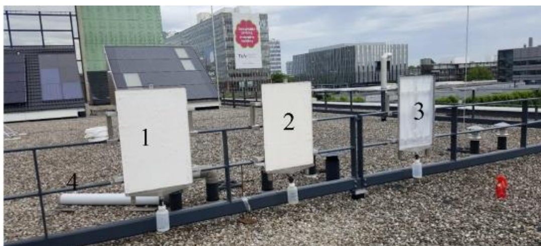
Figura 31. 1: Pannello per intonaco a calce PCO (photocatalytic oxidation), 2: Pannello di riferimento, 3: Pannello in policarbonato PCO (photocatalytic oxidation)
