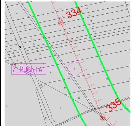
— ELETTRDOTTO AEREO 380 kV IN PROGETTO
