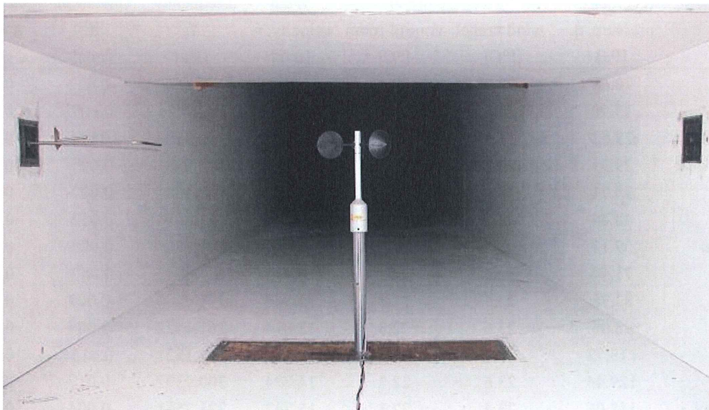
Photo of the wind tunnel setup ( h \times b = 0.85 \times 1.75 m). The shown anemometer is of the same type as the calibrated one.
