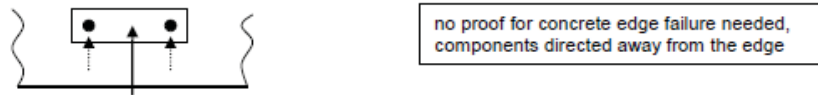
a) group of anchors at an edge loaded by V_{sd} with an angle \alpha_v = 180^\circ
