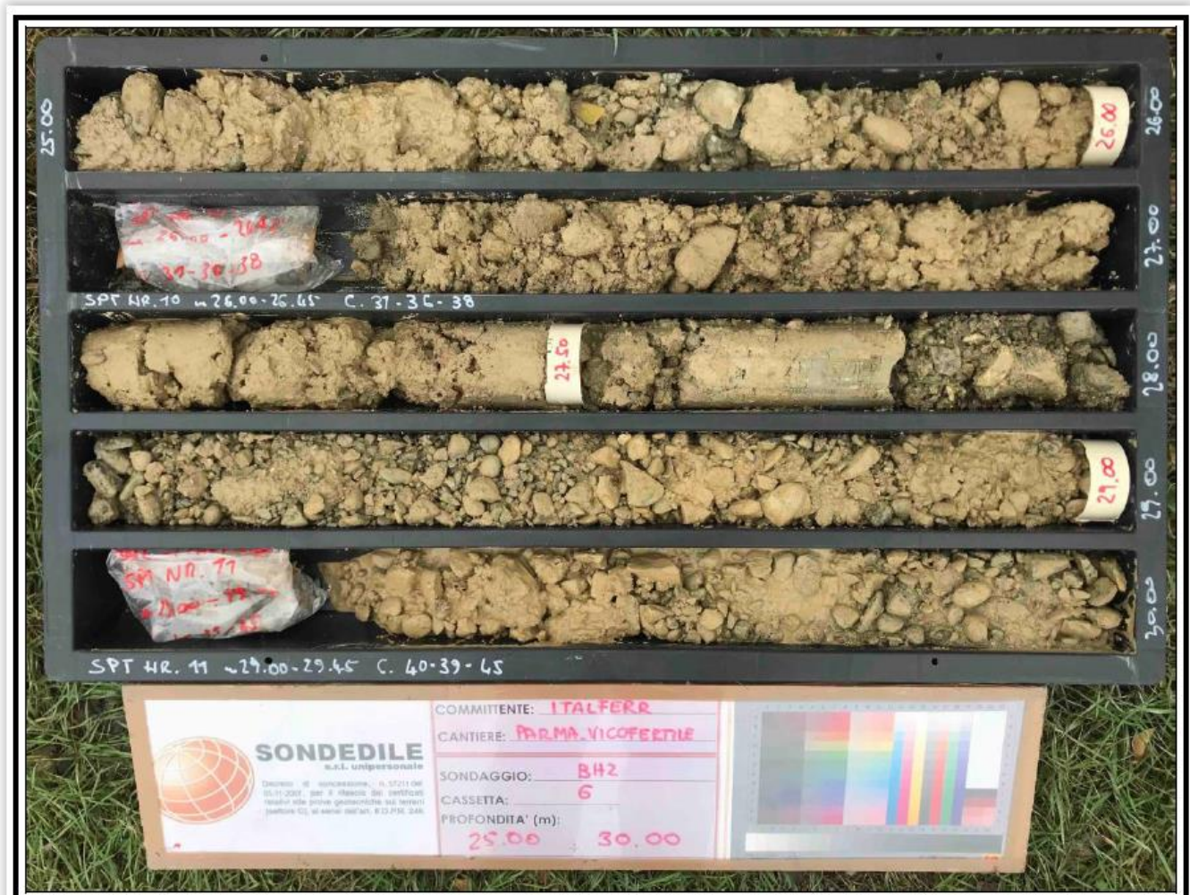
Figura 6-3 – Sondaggio geognostico BH2, litofacies "Ghiaia", 25.00-30.00 m
