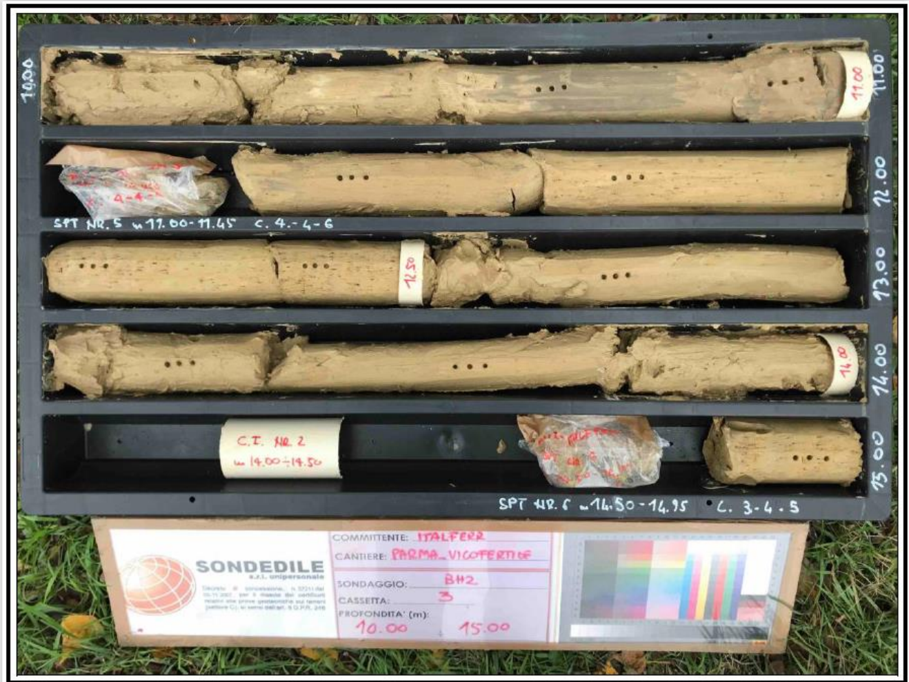
Figura 6-5 - Sondaggio geognostico BH2, litofacies "Limo Argilloso", 10.00-15.00 m
