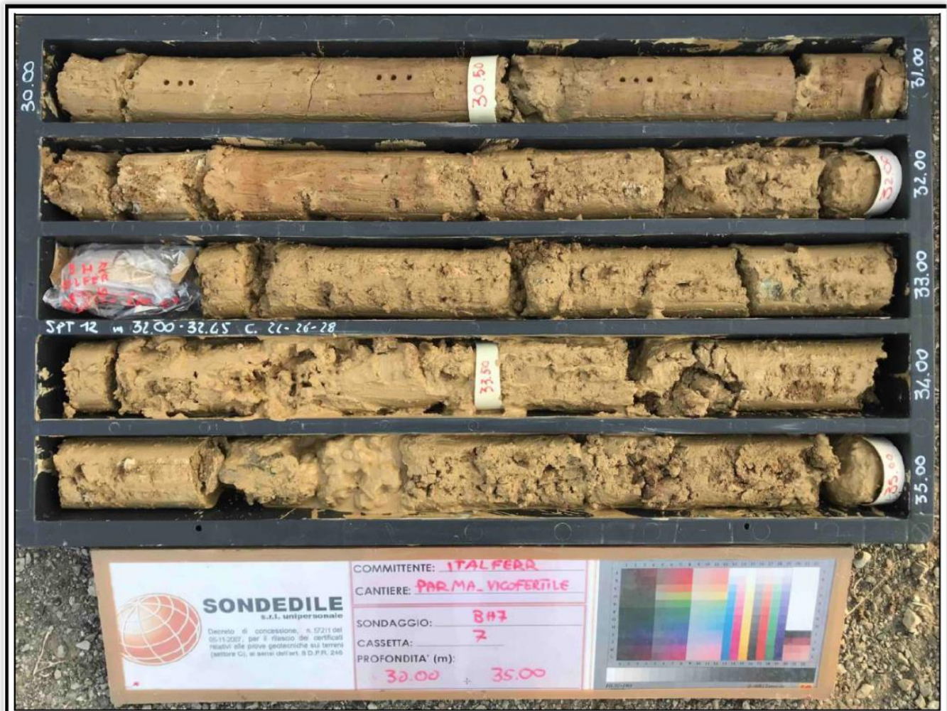
Figura 6-4 – Sondaggio geognostico BH7, litofacies "Sabbia", 30.00-35.00 m
