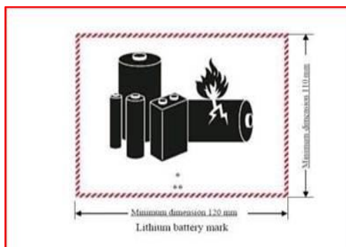
Figure 4 lithium battery handling label
