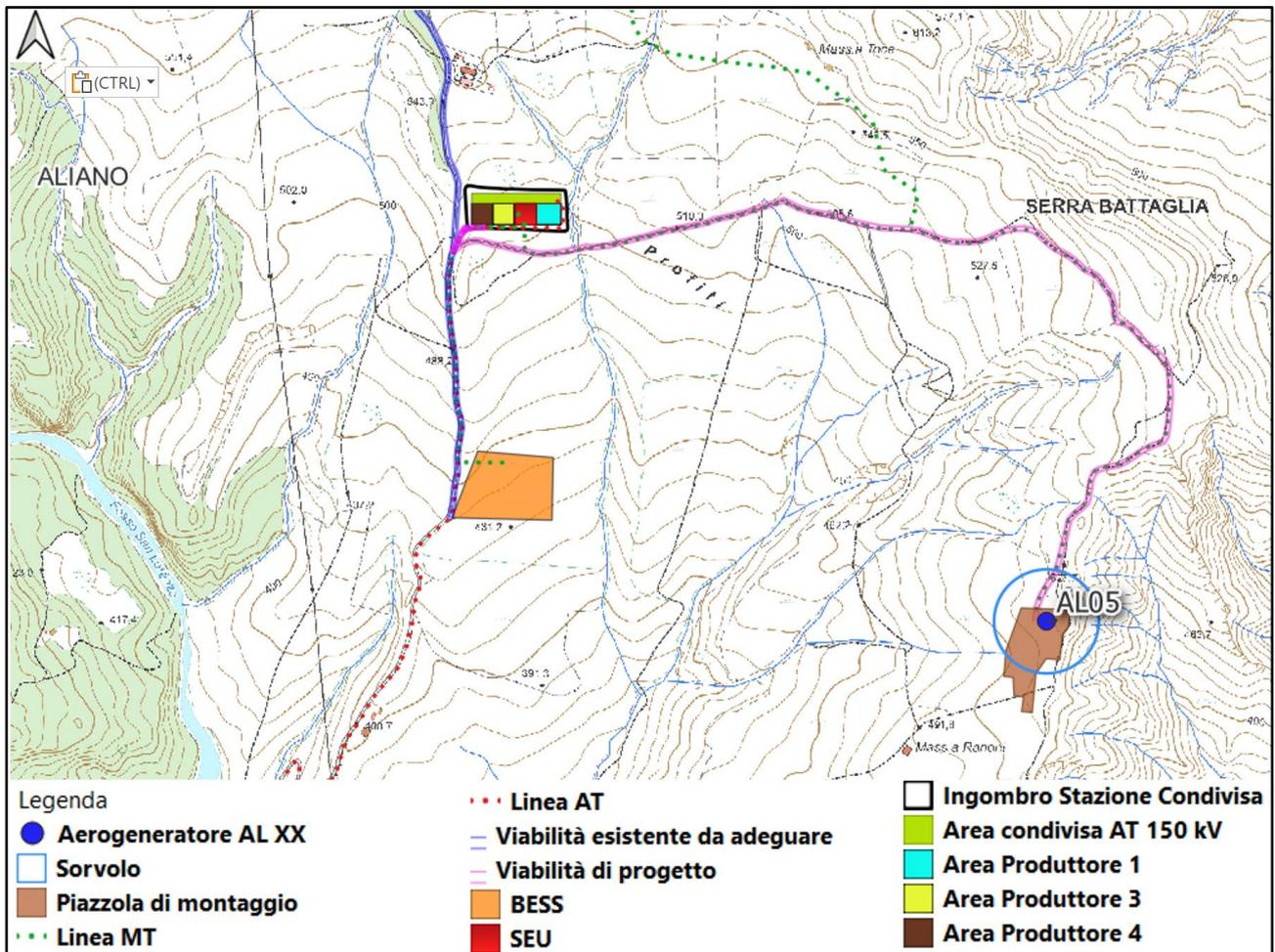
Figura 3.3: Area SEU 150/33 kV e BESS 14 MW
