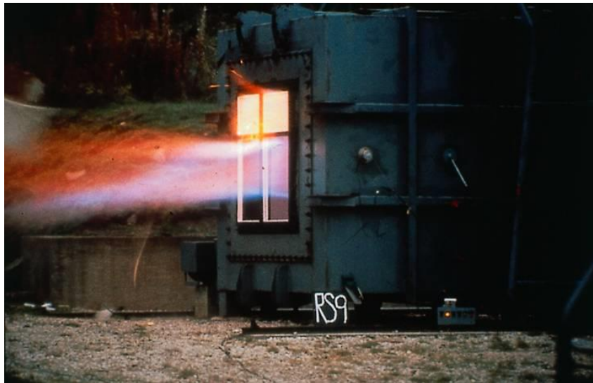
Figure 1: Confined Explosion Showing Venting Combustion Products
