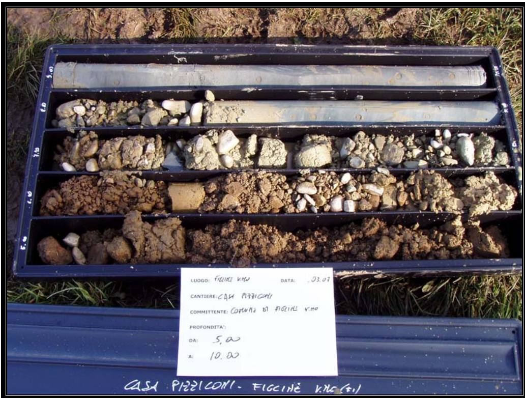
Sondaggio 10 – Cassetta catalogatrice n 2 (5,0 – 10, 0 m da p.c.)
