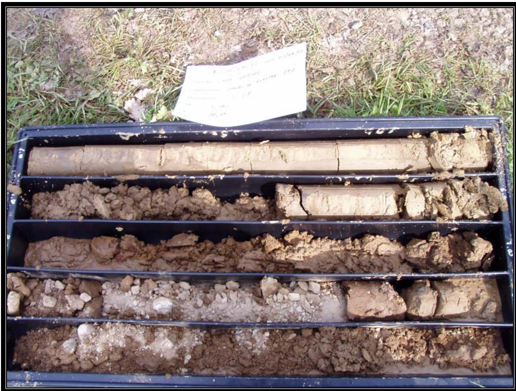
Sondaggio 28 – Cassetta catalogatrice n 2 (5,0 – 10,0 m da p.c.)
