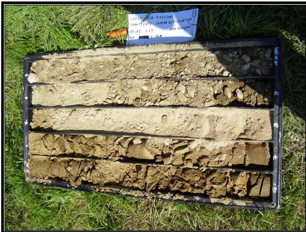
Sondaggio 29 – Cassetta catalogatrice n 2 (5,0 – 10,0 m da p.c.)
