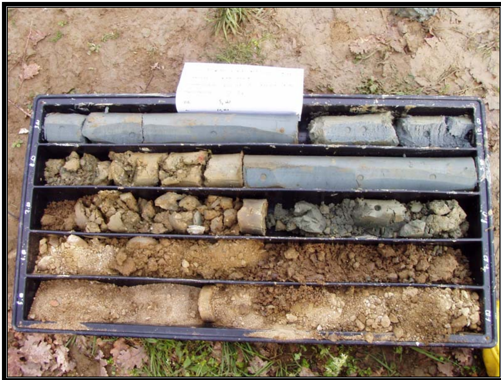
Sondaggio 26 – Cassetta catalogatrice n 2 (5,0 – 10,0 m da p.c.)
