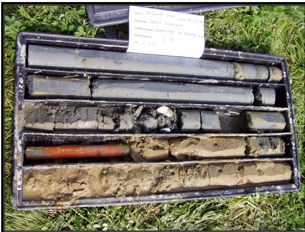
Sondaggio 16 – Cassetta catalogatrice n 2 (5,0 – 10,0 m da p.c.)
