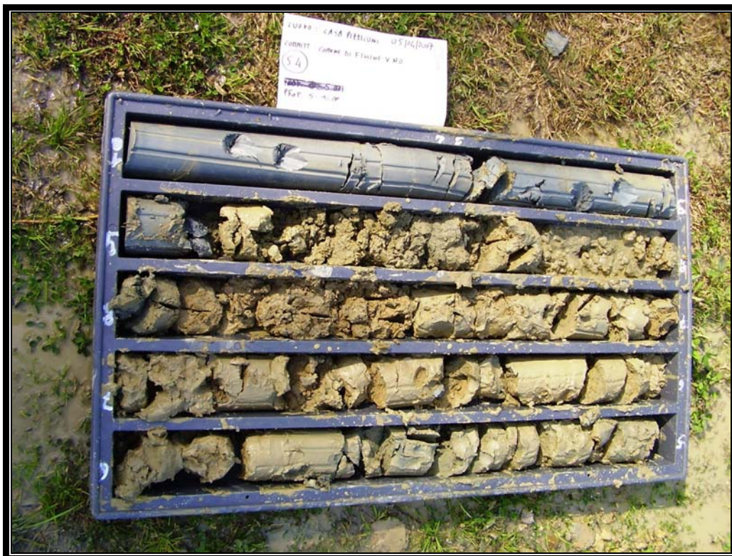
Sondaggio 4 – Cassetta catagolatrice n 2 (5,0 – 10,0 m)
