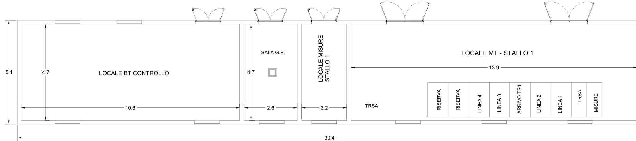
CABINE MT PRODUTTORE e BT CONTROLLO PROSPETTO - NORD
