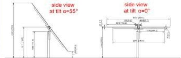
Figure 3-4. Side view of the tracker at two different pitch positions. All measures are reported in mm (model scaled dimensions in squared brackets).
