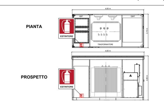
CABINA DI RACCOLTA CON DETTAGLI PREVENZIONE INCENDI (SCALA 1:50)
