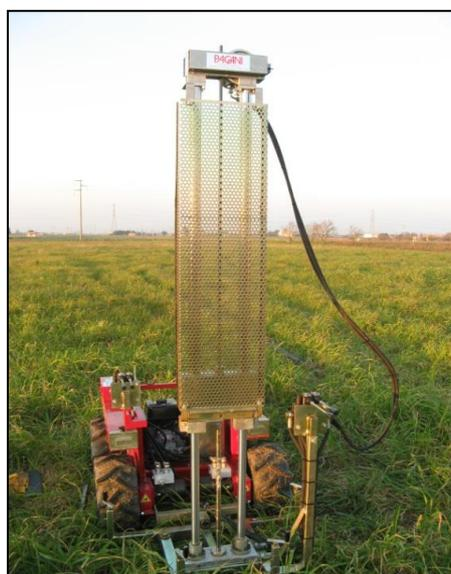
Fig.11: Penetrometro dinamico continuo (DPM – PAGANI Geotechnical Equipment)
