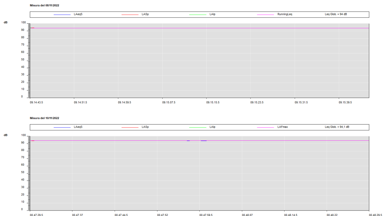
Fig. 7: Taratura Fonetrieche Ante Operam – Cal. 94,0 dB - Taratura Fonetrieche Post Operam – Cal. 94,1 dB
