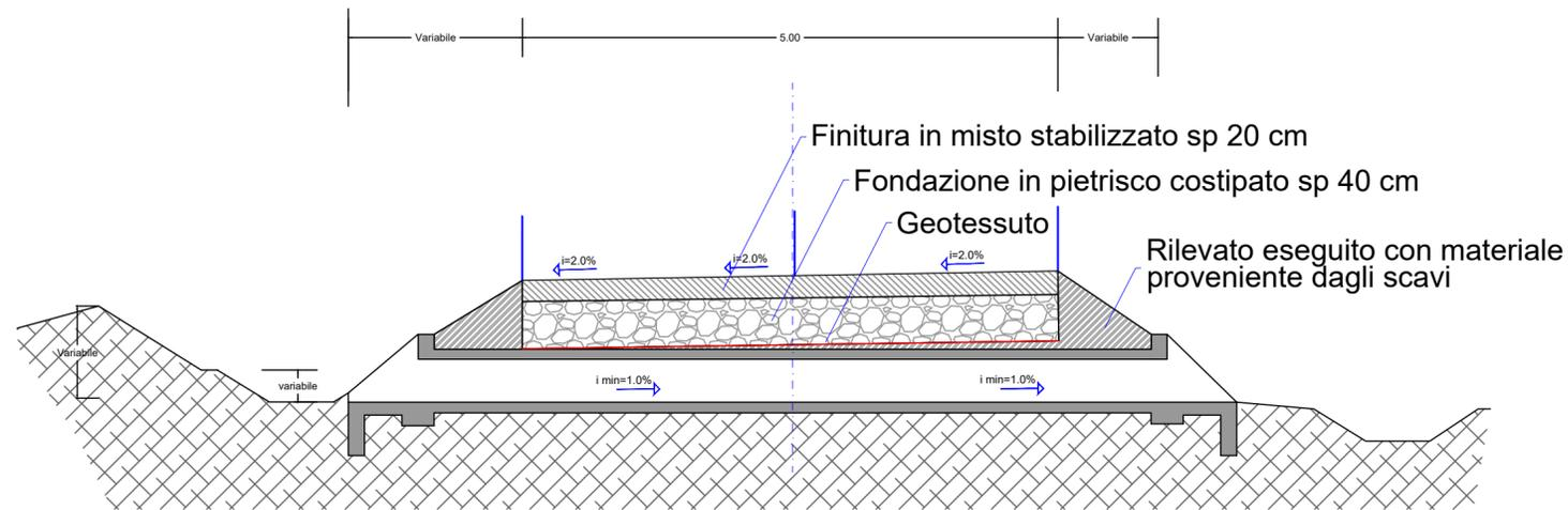
DETTAGLIO MANUFATTO IMBOCCO/SBOCCO\_SCALA 1:50
