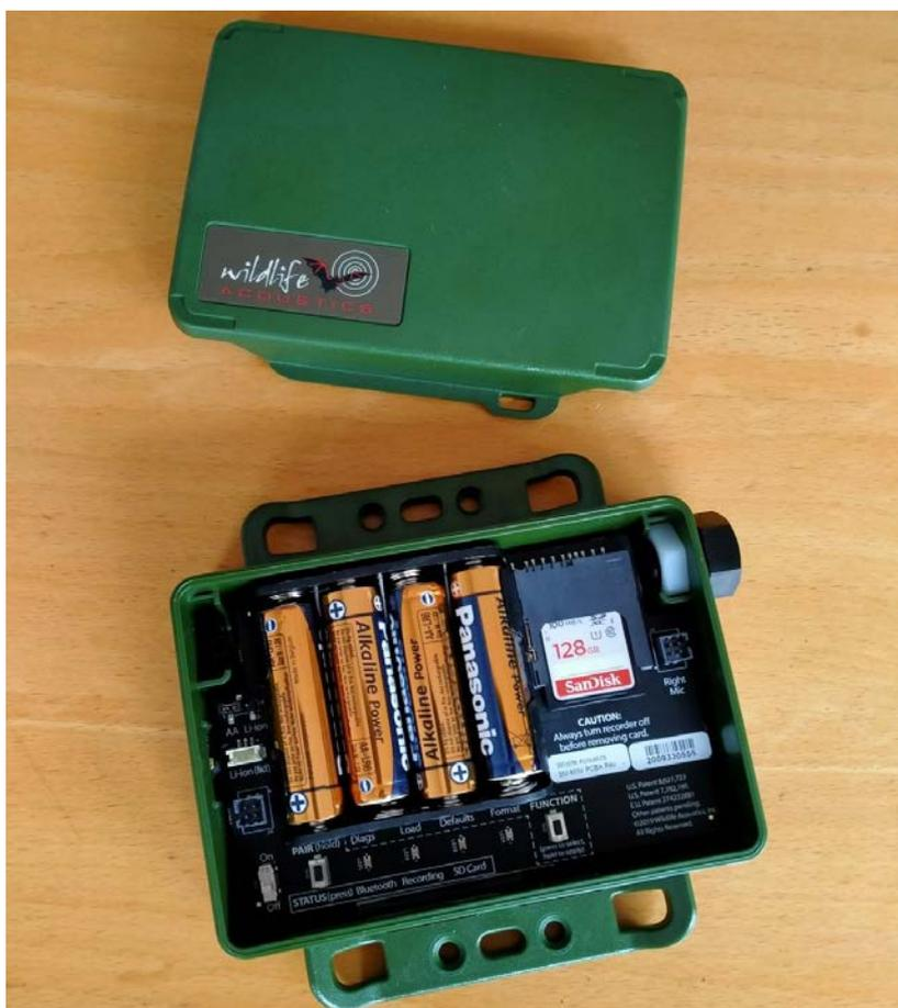
Figura 2.4/C. Bat detector Song Meter Mini Bat Ultrasonic recorder della Wildlife Acoustics
