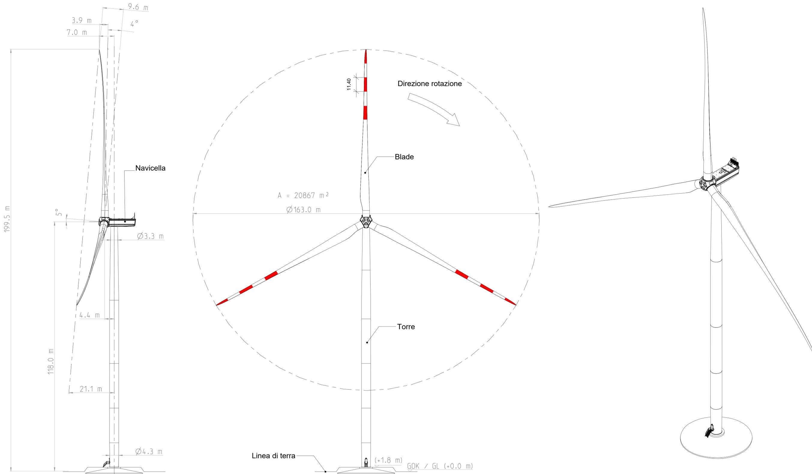
AEROGENERATORE TIPO DI PROGETTO - NORDEX 163
